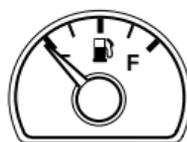
position). The fuel gauge may vary slightly when the vehicle is in motion or after refueling. The ignition should be in the OFF position while the vehicle is being refueled. When the gauge first indicates empty, there is a small amount of reserve fuel in the tank. When refueling the vehicle from an empty indication, the amount of fuel that can be added will be less than the advertised capacity due to the reserve fuel.
