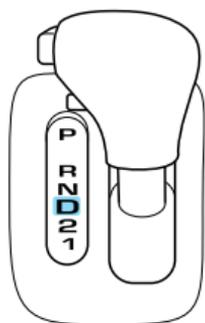
**D** (Overdrive) can be deactivated by pressing the transmission control switch on the gearshift lever.
